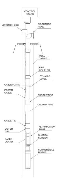
MOTORS: Uses NEMA standard coupling motors designed for continuous use under any effort allowed by its operating curve.
