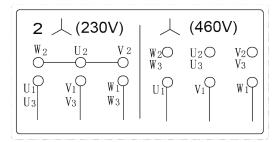
Three-phase connection diagram for models rated 10 HP and above.
