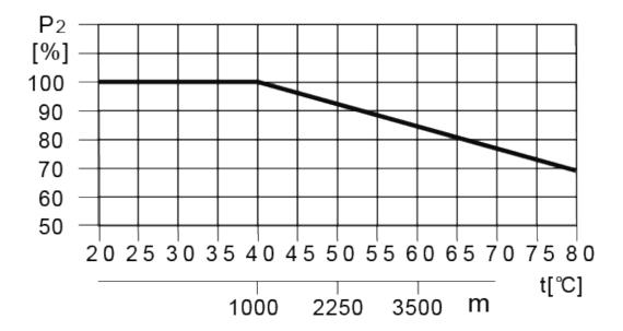
From the previous figure, if the motor pump is installed at an altitude of 11,483 feet (3500 meters), P2 will decrease to 88%. However, if the ambient temperature rises to 158°F (70°C), P2 will decrease to 78%.
